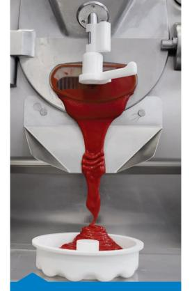
Thanks to the **spacer**, which can be mounted at any time, it is possible to reduce the door opening, thus facilitating the extraction of the Crystal product and the washing of the machine.
