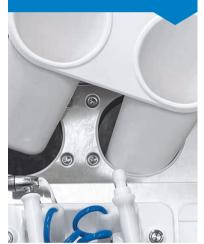
The delayed cleaning program guarantees hygiene by controlling the temperature of the cylinder once the gelato has been extracted. So immediate washing of the machine is not necessary in the event of prolonged work stoppages.
