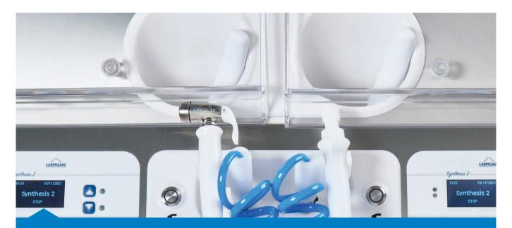
LCD display. Allows the operator to know the operationals status of each cylinder at any time. During the batch freezing process the screen will show:
